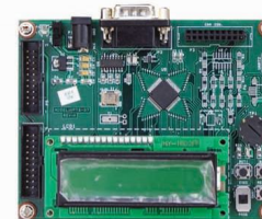
LPC 2148 Project Board
